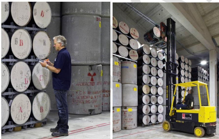
Figure D.5 Low level and intermediate level radioactive waste stored in the LOG.
