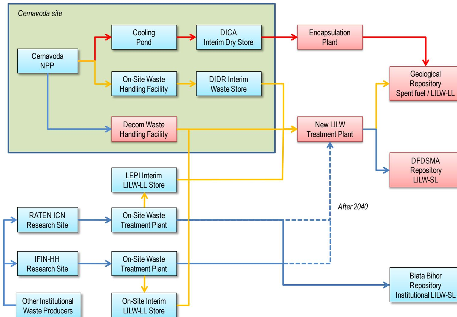
**Figure 2:** An indicative representation of the flows of the different classes of wastes from the main waste producing sites to the final disposal facilities. Red arrows are spent fuel; yellow arrows are LILW-LL; blue arrows are LILW-SL. The red boxes are infrastructure that is planned but not yet built, subject to further approvals
